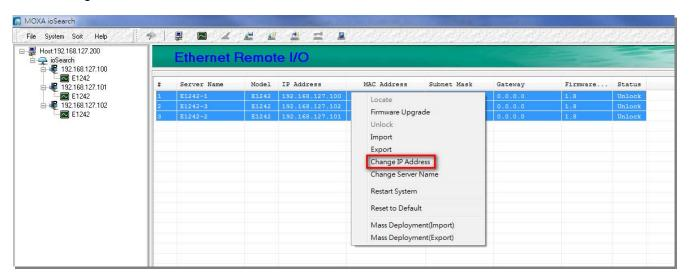
The following screenshot shows the window used to modify IP addresses, subnet masks, and gateways. Users can modify each item and then click "Set" to confirm the modification, or click the "Advance" button to automatically assign IP addresses incrementally.
