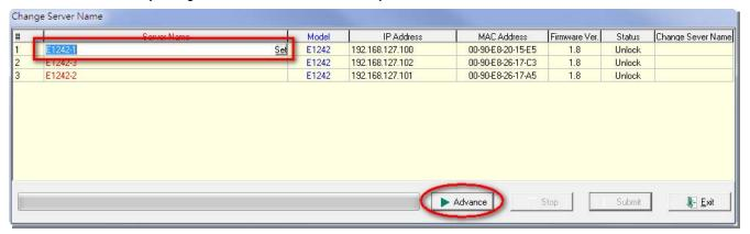
When the following window appears, enter keywords, such as model name, IP address, and MAC address that will be part of the server name. ioSearch will automatically look up the keywords and use those words as part of the server name of the selected devices.
