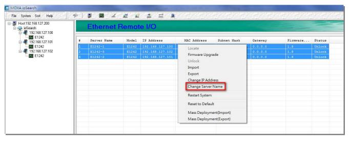
Change the server name of selected models and click "Set" to confirm the modification, or click the "Advance" button to automatically assign server names incrementally.
